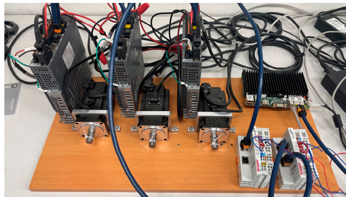
Figure 6. Environment picture of the EtherCAT Master using Python-based real-time control system.
